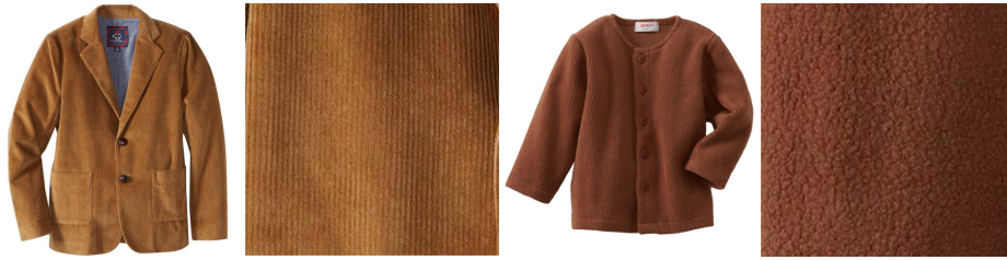
Fig. 1. Different scales reveal different characteristics of textiles. In this case, the micro scale exposes more discriminative features. Columns 1 and 2: Corduroy. Columns 3 and 4: Fleece.
